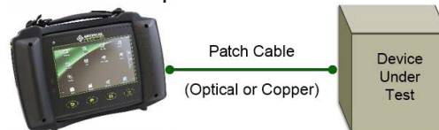
Figure 90 – C37.94 Interface Connection
