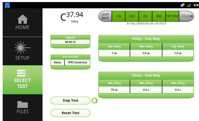
Figure 116 - One-Way Delay Test Results View
